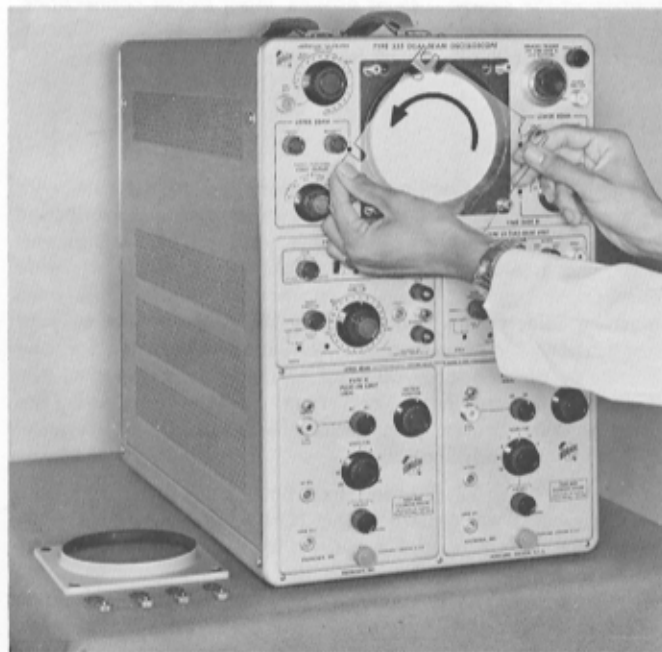
Fig. 2-2. Rotating the graticule to change the color of the graticule markings from red to white or from white to red.
